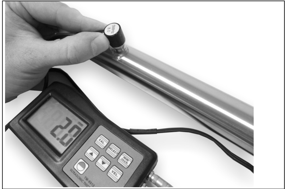
Fig. 2 measure the pipe thickness
