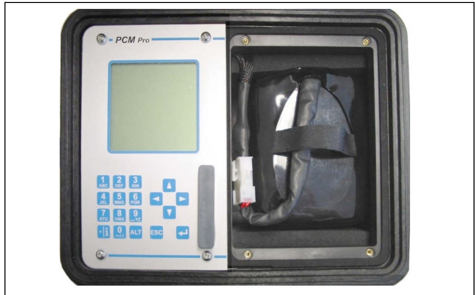
Fig. 8-7 Rechargeable Battery inside of PCM Pro
