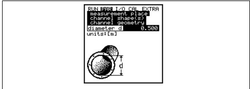
Fig. 10-34 Setting the channel geometry in pipe profiles
