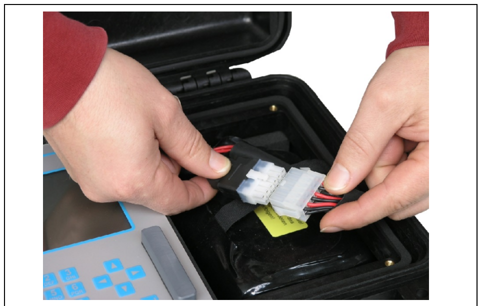
Fig. 8-6 Connection Rechargeable Battery
