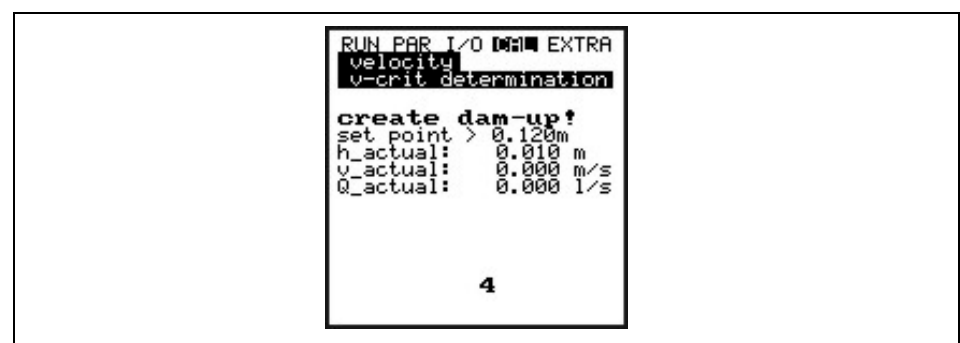
Fig. 10-123 Measuring countdown for the second measuring
