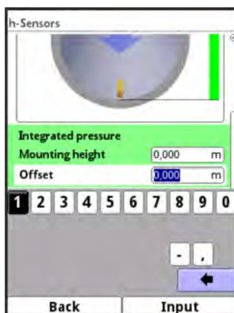
Fig. 39-17 Setting Parameters of the integrated Pressure Sensor
