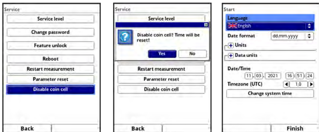
Fig. 42-12 Disable Coin Cell / Putting the Transmitter back into Operation
