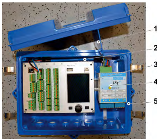
Fig. 21-3 Cable Routing in the Field Enclosure
