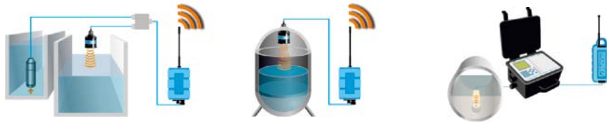
Example: Ultrasonic level measurement in Ex zone, data logger and GPRS transmission
