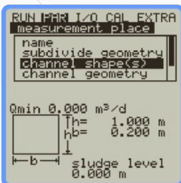
Channel profiles can be set up easily and directly on the unit.
