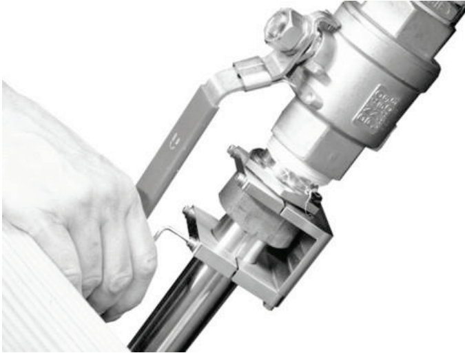
Fig. 13-36 Attaching the final clamp element
