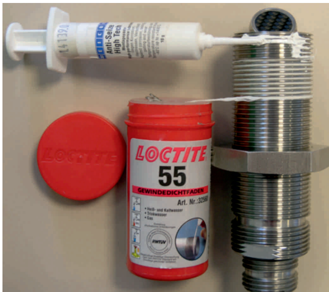
Fig. 13-56 Preparation for installing screw-in sensor
