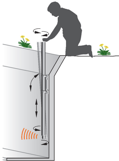
Fig. 14-5 Sensor alignment of rod sensors horizontal and vertical
