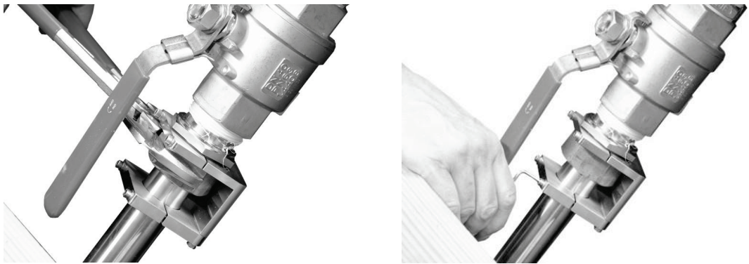
Fig. 13-39 Lock the sensor again after reinstallation
