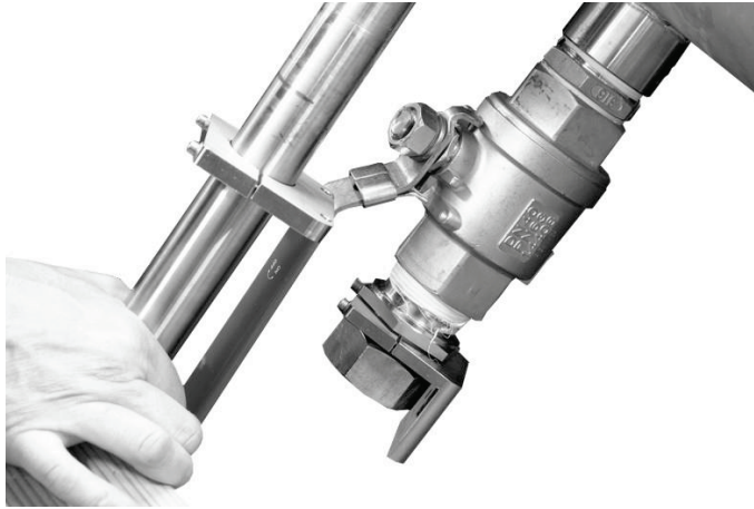
Fig. 13-38 Removing the sensor (maintenance/control)
