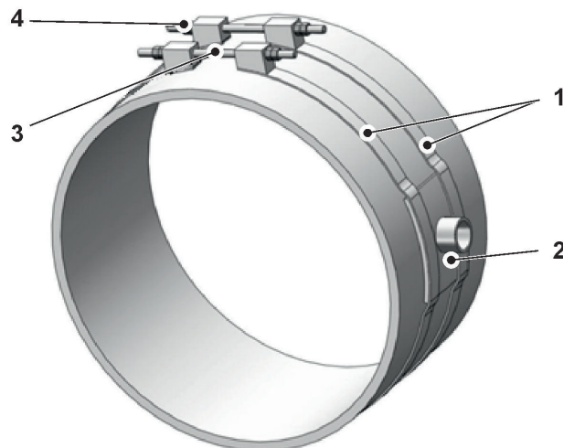
Fig. 18-2 Installation example with tapping saddle DN100...DN400
