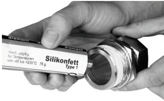
Fig. 13-30 Greasing the sensor screw connection
