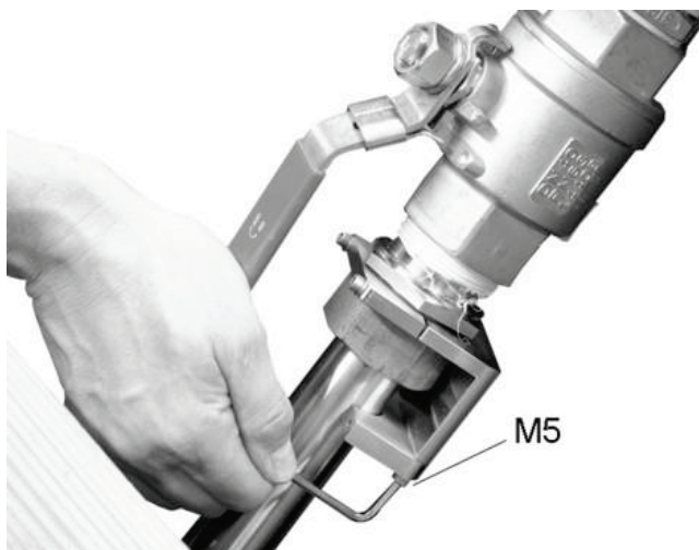
Fig. 13-35 Connecting upper rear and upper front clamp element
