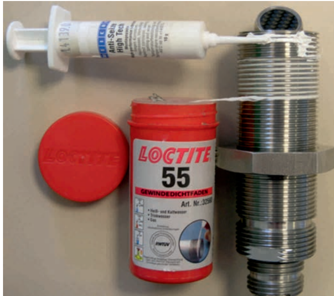
Fig. 10-56 Mounting preparation screw-in sensor
