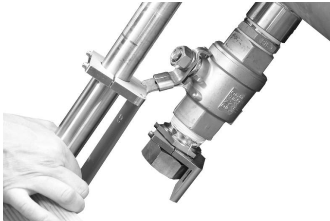
Fig. 10-38 Remove sensor for cleaning and checking
