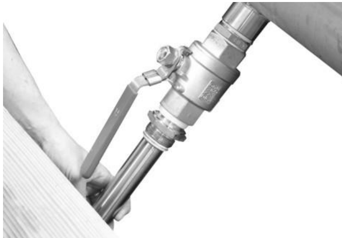
Fig. 10-32 Positioning the sensor
