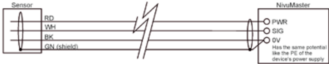
Fig. 19-8 Lines without overvoltage protection
